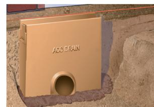
Access or sump unit must be fitted in order to allow subsequent access for maintenance and cleaning. If outletting from access unit knock out pre-formed outlet from the inside, fit PVC-U Ø110mm union, connect to outlet drainage pipework and position on C14/15 concrete bed. If installing sump unit follow above steps from fit PVC-U Ø110mm union.
