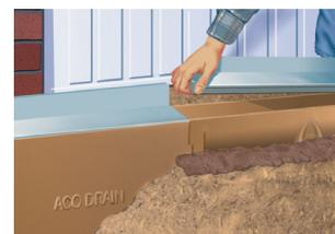
With Brickslot covers fitted haunch around channels with concrete. Bricks/paviours should be laid in Epoxy or Polymer Modified Mortar for lateral stability. Final surface to be 3-5mm above slot.
