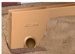
Lay channels starting from sump/access unit, ensuring joints connect by lowering units horizontally. Fit endcap to end of channel. For fully watertight joints, use a suitable sealant (contact a sealant specialist for guidance).
