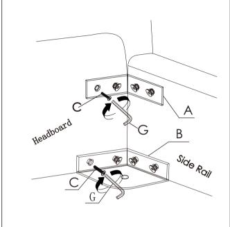
Attach side rails to headboard with part A, B using C bolts.
