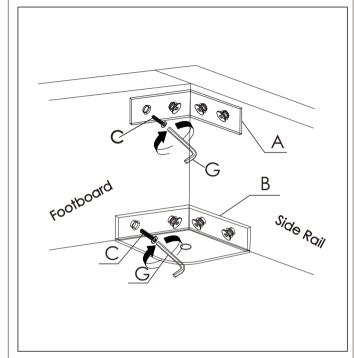
Attach side rails to footboard with part A, B using C bolts.
