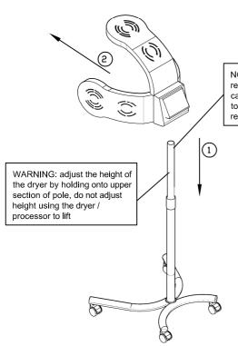
NOTE: Screw needs to be removed from top of pole, carefully lower Horizon Processor top onto pole, line up holes and replace screw to secure.
