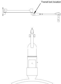
6. Once the Dryer or Processor is in position it is safe to remove the Transit Lock. To accomplish this, gently pull down the Lower Arm (front section) until there is no pressure on the Transit Lock, thus enabling easy removal. (Always keep Transit Lock in a safe place for future use. NEVER REMOVE the Dryer or Processor from the Arm, without first TURNING OFF THE POWER and re-locating the Transit Lock.)
