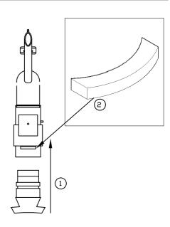
3. Insert Swivel Boss of Dryer or Processor into Pivot Hood [1], lining up the groove in the Boss with the slot in the Hood and place the Locking Wedge in position
