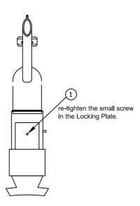
5. Rotate Dryer or Processor to check that it turns smoothly through 360 degrees before re-tightening screw in Locking Plate [1]. The Locking Wedge is now held securely, preventing the Dryer or Processor from dropping out of the Pivot Hood.
