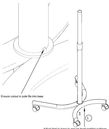
Adjust feet to base to ensure level working surfaces.
