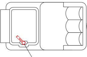
Recommended fitting of tap at 45 degree angle to allow added space for client
