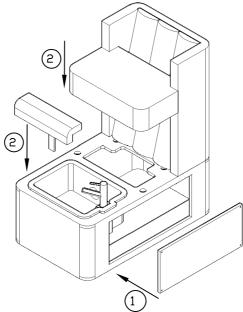
6. Connect unit to on-site power supply. Replace side access panel [1].
