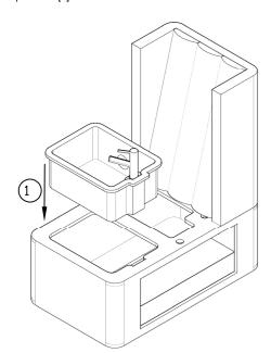
5. Carefully lower Basin (D) into position [1] The basin must be bedded on Silicone Sealant (not provided), and fully sealed before use.
