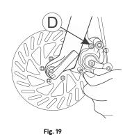
To install new pads, remove the brake caliper from the fork or frame by unscrewing hex bolts D (Fig. 19). Unscrew (left/counterclockwise), the smaller hex bolt inside allen bolt B (Fig.14). Lift up and pull the inner pad downward, using the protruding tab. Slide a thin slot screwdriver under the outer pad and lift it up. Hold the screwdriver in this position and remove the pad with a pair of long- nosed pliers.
