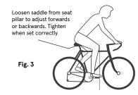
The saddle should be moved forwards or backwards so that the knee is directly above the pedal when crank is parallel to the ground
