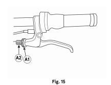
Tighten the Locking Collar up to the lever body. Additional adjustments at the caliper (Fig. 16).
