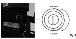
From the initial 12 o'clock position (battery and carrier are unlocked), insert the key into the key slot, press and turn it clockwise to 6 o'clock position (battery now locked into the housing). Reverse steps to unlock.
