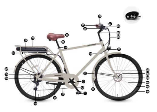
Fig. 1 Electric Bicycle with Carrier Pack
