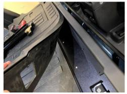
Align the locating pegs in the Defender trim with the holes in the underside of the trim panels.
