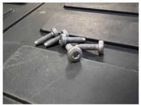
Where the return lip of the trim sits flat onto the floor of the Defender loadspace, fix into the wooden floor panel using the supplied self-tapping screws.
