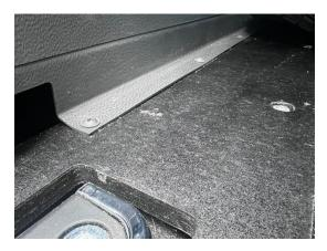
Tighten down the M6 Torx fasteners behind the seats.
