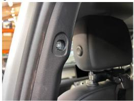
Locate the plastic blanking plugs into the recess and fasten using some of the M6 Torx fasteners you saved when removing the bulkhead. Note that there are two different shapes of blanking plugs that fit the upper and lower fixing locations.
