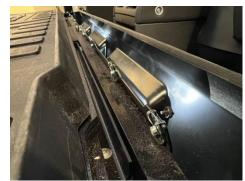
Lift up the front edge of the loadspace matting. The rearmost edge of the finisher trim sits on the Defender floor underneath the front edge of the matting.
