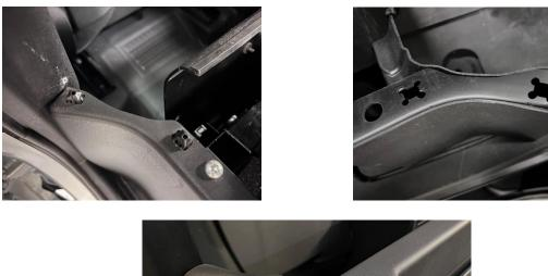
With the LH & RH trim finishers in place secure the front face of the trim behind the seats by re-using some of the grey coloured M6 Torx fasteners you've removed when removing the bulkhead and trim pieces. Start each fastener in the Chimney nuts but don't tighten them fully until they are all in place.
