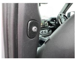
Alternatively, you can install the factory fit Grab Handles (available in the MUD store) onto the B Pillar that are used on the regular Defender models with rear seats. The handles can provide an occasional lashing point for securing larger loads.
