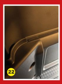
Slide an M6 Chimney nuts onto the plastic tab (circled in yellow) on the B-Pillar in the pics on both Left and Right hand sides of the car.
