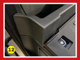
Slide the M6 Chimney Nuts into place over the slotted holes in the upright tabs on the steel panel behind the seats. Note that the left and right hand sides of the bulkhead finisher use a different number of fasteners.
