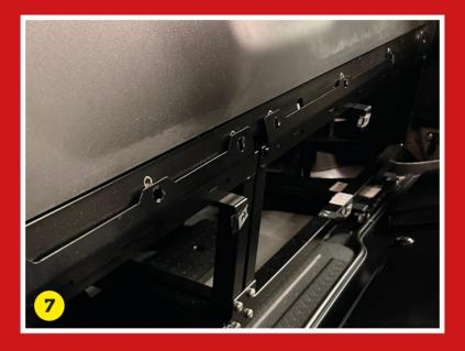
From the front cabin of the vehicle remove the 8mm headed bolts (3 per side) that secure the bulkhead to the pillar support brackets.
