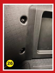
Finally, secure the top edge of the corner finisher trim using one of the self-tapping screws. Drill a 3mm pilot hole for the screw fixing.
