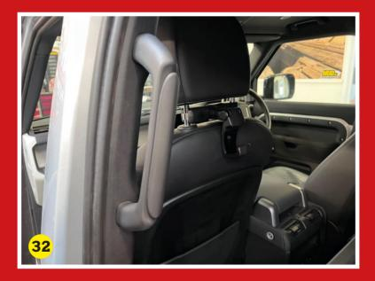
Reuse the longer (black) TX30 Torx fasteners you removed from the metal B-pillar brackets to fix the factory grab-handles.
