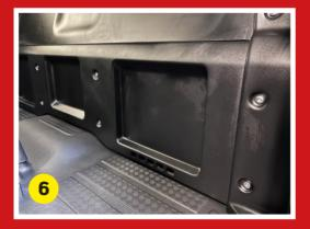
With the plastic trim panel removed this will give you access to the row of 8mm headed bolts that secure the lower edge of then bulkhead into the car. Remove all of the 8mm headed fasteners.
