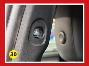
Locate the 3D printed blanking plugs into the recess and fasten using more of the M6 Torx fasteners you saved when removing the bulkhead. Note that there are two different shapes of blanking plugs that fit the upper and lower fixing locations.
