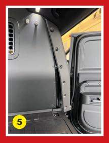
Remove the Torx fasteners running across the full width plastic trim panel immediately behind the front seats.
