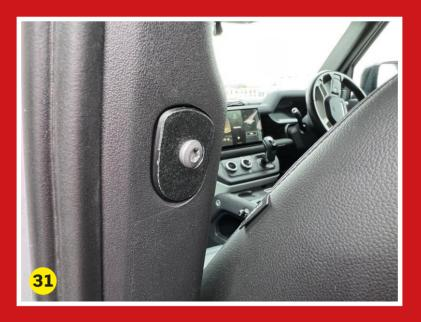
Alternatively, you can install the factory fit Grab Handles onto the B Pillar. The handles can provide an occasional lashing point for securing larger loads. The same part fits both LH & RH sides. A Grab-Handle kit is available to buy from MUD-UK.
