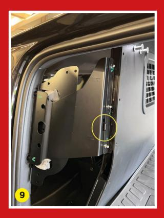
Even with all 6 of these bolts removed, at this stage the bulkhead will still be held securely in place by the T-shaped metal tab (circled in red in the pic) that hooks into the slotted hole within the B-Pillar brackets.
