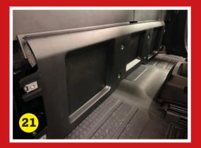
The kit for the 90 models includes a pair of additional corner finisher trims for the lower B-Pillar area. They are handed for Left and Right sides. The top corners of the trim sit as per the pic below.
