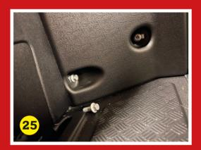
Now use another pair of the Torx headed fasteners to secure the front face of the corner trim.
