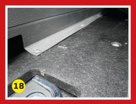
Now tighten down the row of M6 Torx fasteners behind the front seats.
