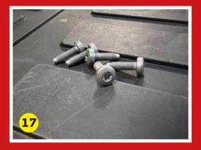
Where the return lip of the trim sits flat onto the floor of the Defender loadspace, fix into the wooden floor panel using the supplied self-tapping screws. Drill a 3mm pilot hole for the screws.
