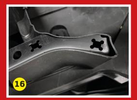
With the LH & RH trim finishers in place secure the front face of the trim behind the seats by re-using the grey coloured M6 TX30 fasteners you've removed when removing the bulkhead trim pieces. Start each fastener in the Chimney nuts but don't tighten them fully until they are all in place.
