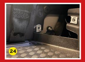
We recommend fixing the corner trims in place by locating the 8mm headed bolts in the B-pillar first.
