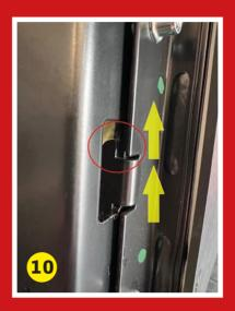
Lift the bulkhead **Upwards** and then **Backwards** to release the T-shaped tabs from the slotted holes.
