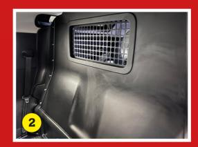
Remove all of the fasteners from the Left & Right Hand B-Pillar trim panels from the loadspace area.
