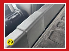
The exposed threaded holes on the B-pillar trim are where the grab-handles would normally fit on a regular passenger car derivative of the Defender 110 & 90.
