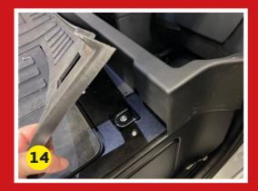
On 110 models align the locating pegs in the Defender trim with the holes in the underside of the trim panels.
