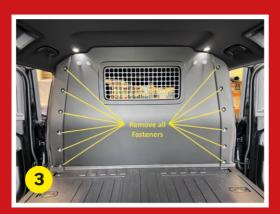
Just like the front trim panels there are additional fixings at the top of the trims that use concealed fir-tree fasteners on the reverse side of the trim. Pull on the upper half of the trims to release the fir-trees.
