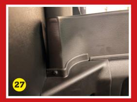
Attach the U-shaped centre trim using the 3M VHRB adhesive sticky pads. We recommend attaching the pads to the Divider and then lowering the U-shaped finisher trim over the top of the trim.
