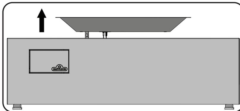
3. Remove the burner from the enclosure. Take care not to damage or kink the thermocouple wire.
