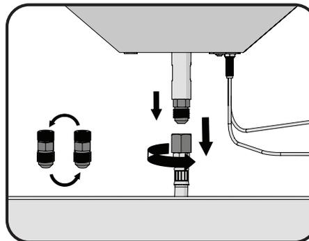
6. Replace the propane orifice with the natural gas orifice supplied. Note: The air shutter has been factory set and does not need to be adjusted.
