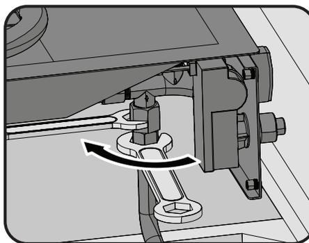
4. Disconnect the stainless steel flex connector from the orifice using (2) wrenches.
