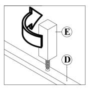
Attach Center Rail (D) with Extra Leg (E) to bed. Please DO NOT attach Center Rail (D) without first securing Extra Leg (E) to the whole body otherwise Center Rail (D) might break. ASSEMBLY IS COMPLETED
