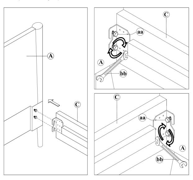
3. Attach Footboard (B) to the components.3.1. Please note the indicating letter for homing guidance.3.2. Please hang the brackets to the Hexagonal bolts (aa) and tighten by using Wrench (bb) (see below diagram).
