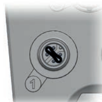
Fig. 18: Conductive rubber band in connection socket 1
