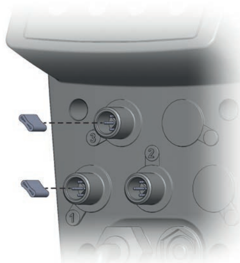
Fig. 16: Conducting rubber hoses in the connections 1 and 3 of the MAGDOS LA/LD
