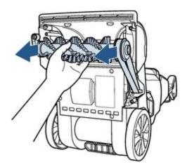
• Remove belt off motor shaft
