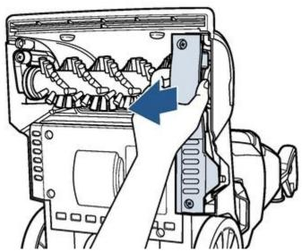
• Pull brush roll out and remove the belt from track
