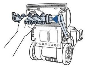
• Align the brush roll mount with the screw post
