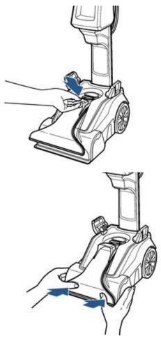
• Return dirty water tank to machine, secure with latches
