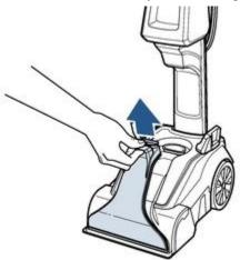
• Rinse nozzle under water and wipe debris from machine where nozzle was
