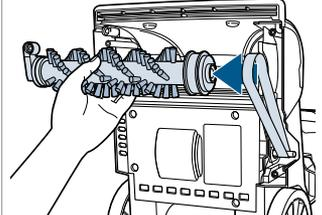
**6.** Put the belt on the Brush Roll track. Put the Brush Roll back into position.
