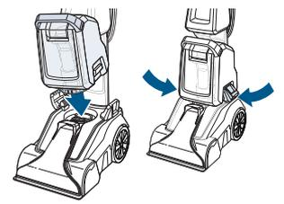
**9.** Once Dirty Water Tank is dry align the bottom of the tank to the base and secure into place with latches.
