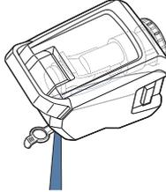
**5.** To empty, pour out dirty water using opening at back of tank. Rinse the tank thoroughly. Reinsert tab into tank.
