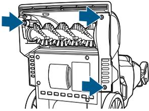
**1.** Turn OFF and unplug your machine. Use a Phillips-head screwdriver to remove the 3 screws.
