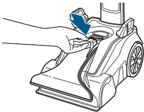
**7.** To replace the Nozzle, align top into channel in front of red filter and press in place.
