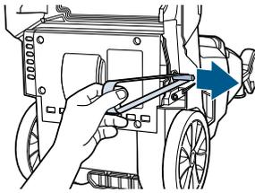
**4.** Pull belt off of motor shaft.
