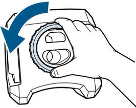
**4.** Ensure the Dirty Water Tank is empty by gently removing the float stack and unscrewing the ring at the bottom of the tank.
