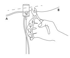
**A.** Route the electrical wire through the large holes in the cable holders.
