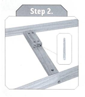
Attach one of the timber blocks part #5 using four of the screws from (Bag B). \*NOTE: Make sure the side hole in part #5 is facing the center of frame. Add small brass pin from (Bag D), into the side hole of part #5 that is attached to frame. (As shown in picture to the left)
