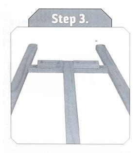
Slide part #4 onto the small brass pin from (Bag D), making sure that the angled cut is facing the frame. Screw remaining part #5 onto frame with remaining screws from (Bag B).
