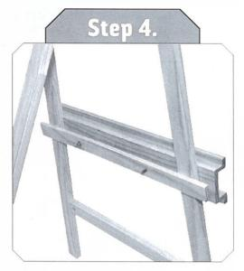
Adding parts #1 & #7, to frame using contents from (Bag C). Making sure part #7 is between part #4 and frame.
