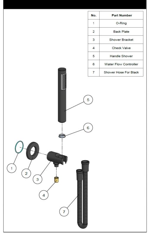
NOTE: The hose end caps of parts (hose part 7) are made from a special hardened plastic to prevent the brass mount (3) from scratching.
