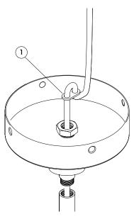
To adjust the height, remove the cable from the Ceiling rose (A).
