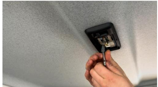
Note: Some of the fixings may shear on removal. If this happens they can be removed with pliers. Plastic trim tool is recommended as the likelihood of scratching the lens is reduced.
