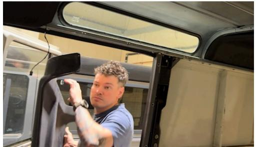
Note: Some of the fixings may shear on removal. If this happens they can be removed with pliers.
