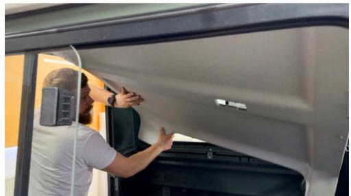
Note: Some of the fixings may sheer on removal. If this happens they can be removed with pliers.
