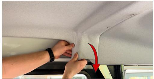
Once the headlining has been removed, this can now be taken out of the rear tailgate door.
