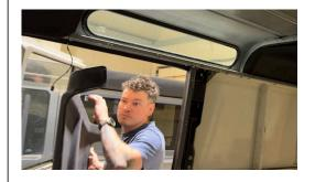
Note: Some of the fixings may sheer on removal. If this happens they can be removed with pliers.
