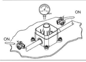
Turn the water on below 0.8Mpa of pressure. Maintain for 30 minutes and check for water leaks.
