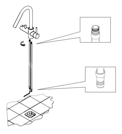
take out the 2 water inlet pipes from the packing box, fasten them onto the spout.
