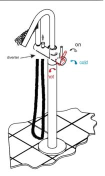
Switch between the spout and hand shower by using diverter.
