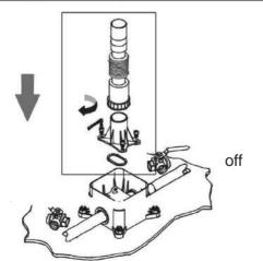
Install the pipe cleaning parts.
