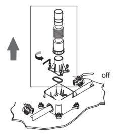
Turn off the valve and remove the pipe cleaning parts.
