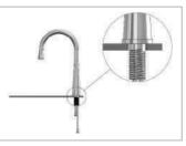
3. Attach the counter weight to the pull out flexible hose (part 2) DO NOT TIGHTEN (as the counter weight will need to be adjusted later on. Connect the flexible hoses and tighten (part 7) to the water outlet ensuring the rubber seal is not missed.
