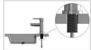
3. Place the rubber washer (part 2) over the flexible hoses and push up until it is firm against the surface being mounted on, then push (part 3 + part 5) the fixing plate and fixing nut over the flexible hoses and tighten firmly and tighten screws where applicable.
