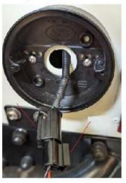
You will now need to route the RCA cable down the length of the vehicle. You will notice the fly leads on the RCA cable that need connecting to the fly leads on the piggy back loom are at the end of the RCA cable which is connected into your head-unit. You will therefore need to extend the red and black fly leads from the piggy back loom to the front of the vehicle to connect into the +VE (red) and -VE (black) wires this provides the trigger for the camera.
