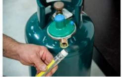
**3.** Connect the flexible hose to the pressure regulator.
