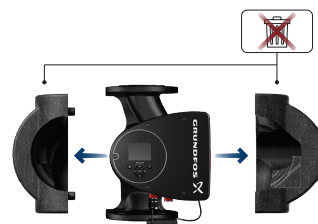
Removing insulating shells from the pump
