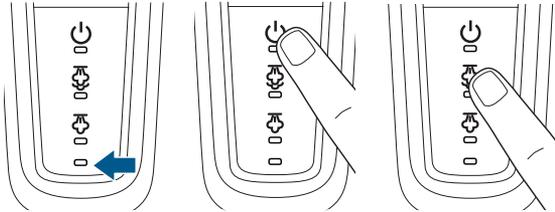
Plug the machine into a properly grounded outlet. Once the blinking READY light turns solid, press the POWER button. Next select the appropriate steam level.
