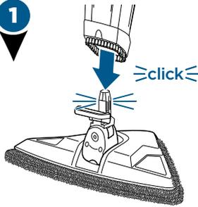
Attach lower body to mop head by snapping it into place.
