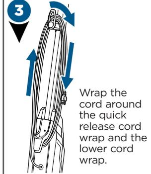
**NOTE:** To easily unwrap the cord for use, just turn the quick release cord wrap downward to remove the cord from the cord wrap.
