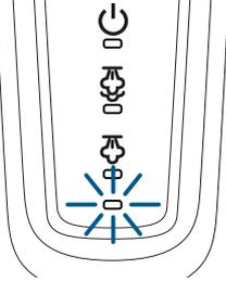
Plug machine into a properly grounded outlet. The READY light will begin blinking. The blinking light indicates the machine is warming up.
