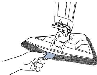
Turn off and unplug the machine from the grounded outlet. Carefully remove mop pad using the Quick Grip Release Tab from the mop head.
