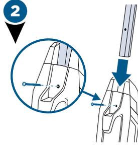
Then, insert handle into body of unit and screw until tightened.
