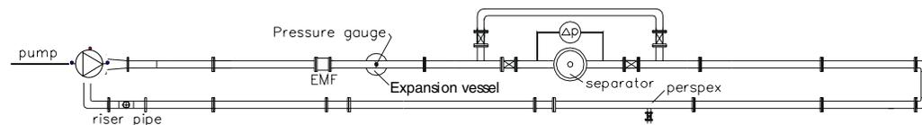
The riser pipe is closed to establish a pressure of 3.0 bar abs.
