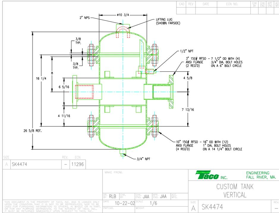
Figure 2: Taco air and dirt separator 4903AD-4 (prototype)
