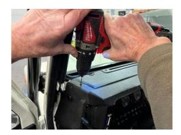
Drill through the holes in plastic end trim into the top rail with a 3mm drill to create the 2 x fixing holes (top & side) that secure the heater control end trim into the dashboard-rail.
