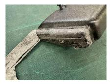
Make a cut line with a sharp bladed knife and peel away the vinyl from the **drivers side** end of the dashboard-rail. Ignore the threaded insert on the drivers side. This is only used for the grab-handle fixing on the passenger side.
