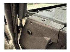
The end of the dashboard rail that tucks under the heater control on the end of the binnacle will need the layer of vinyl trimming back prior to installation to allow the plastic trim to sit neatly over the end of the dashboard rail.
