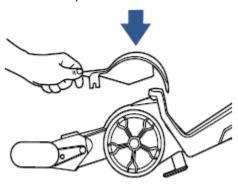
Replace the brush cover and front nozzle to test
