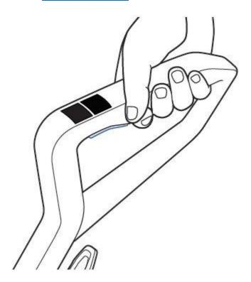
Remove dirty water tank by pressing down on the recessed button on the top of the tank
