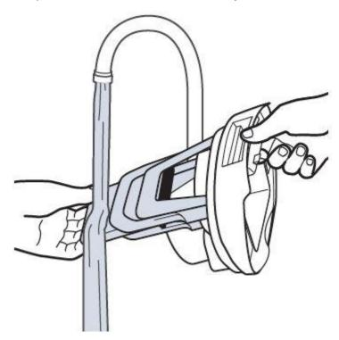
• Replace filter (after it has dried) - be sure the edges are smooth and not folded over
