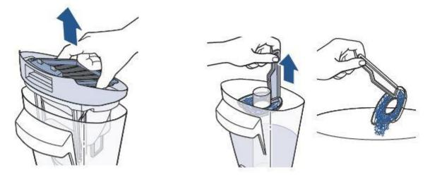
• Remove filter and clean any debris
