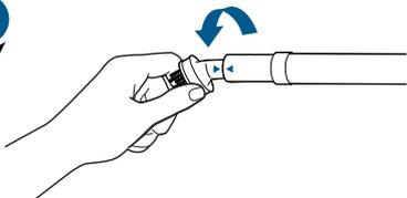
Align arrow on tool to arrow on end of nozzle (on Extension Wand or handheld steamer) and twist tool into place.
