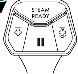
After 30 seconds, the STEAM READY light will turn to a solid light. This means the steam mop is heated and ready to use.
