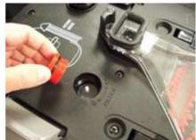
c. Remove the white filter by lifting it out by the post and rinse it under water to clean.
