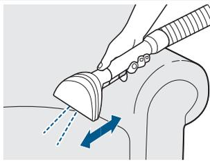
**8.** Hold tool about 2.5 cm above soiled surface. Press spray trigger to apply cleaning solution. Release trigger, apply downward pressure, and pull toward you to suction up dirt and cleaning solution. Do not overwet.
