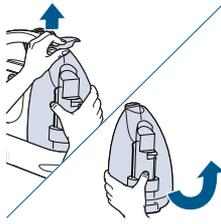
**2.** Empty and rinse the Dirty Water Tank after each use, OR when dirty water reaches the fill line. To remove the tank, lift up the Dirty Water Tank retainer lever.
