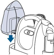
**4.** Replace the tank by lining up the vertical guides on the left side of the machine with the indentations on the tank and slide it down into place.
