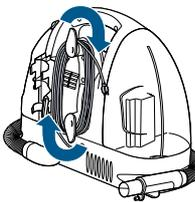
**7.** Wrap power cable around the cable wrap on the back of the Little Green.
