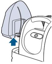
**1.** Remove the Clean Water Tank by lifting it straight up and then away from the machine.
