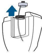
**2.** Unscrew the black cap at the bottom of the tank.
