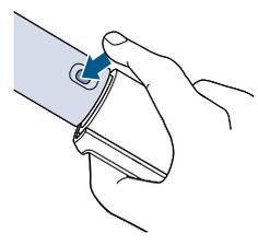
**3.** Disconnect the cleaning tool from the spray trigger by pushing down on button lock and pulling straight off (DO NOT twist tools to remove them).
