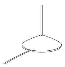
Ensure the cable runs through the prefabricated channel in the base of your Boyd lamp body.
