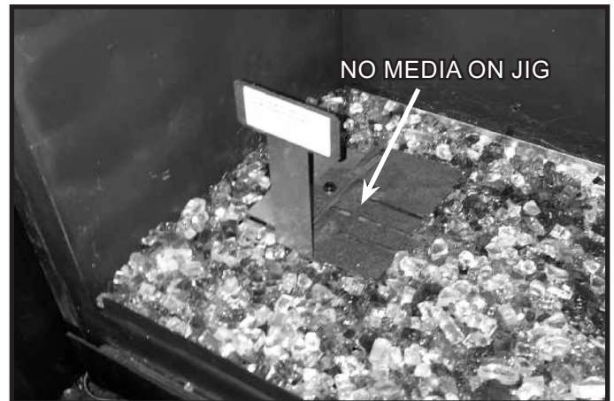
Figure 2. Media Placement Jig in Place
