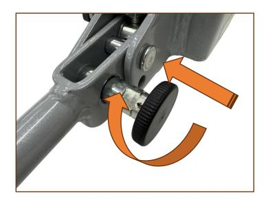
It is possible to tighten the grip on the tow-ball by removing the bracket from the tow-ball and adjusting bolt **B** concealed under the push-on plastic cap.
