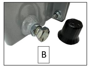
• Undo the lock nut and tighten bolt B a small amount at a time. Remember to re-tighten the lock nut.
