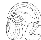
2 When you want to change the cable. please press the small button for release and simultaneously pull off the cable connector from the headphones.
