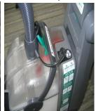
• Machine may have lost prime. To prime, turn the machine off and wait one minute. Turn unit back on and depress the upholstery hose trigger. Check for spray.
