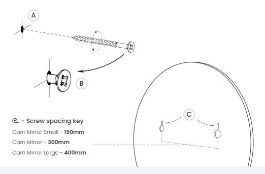
\*\*\* The mirror must be picked up by the glass only. Handling the mirror by the wooden hoop will put strain on the fixing between the glass and hoop and could cause the mirror to fall and the join to break. We also recommend the Carn Mirror Large be installed by two people.
