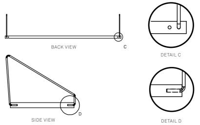
**6.** Hang the shelves (premounted with the brackets) within the screws that are now mounted on the rails. Be sure that the steel bracket rests on the inner screw.
