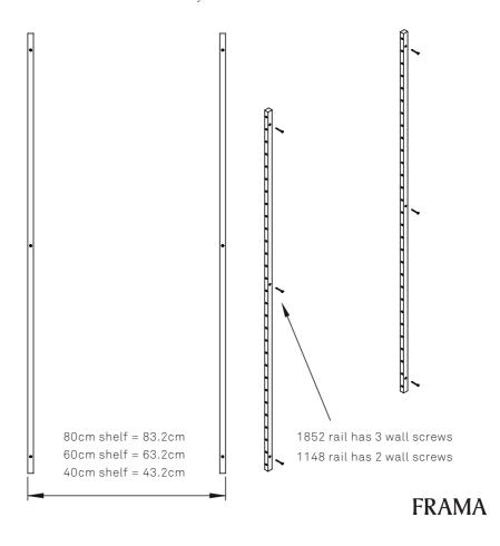
**4.** Fasten the screws and bolts to the heights you want to mount the brackets. Use the same heights on the left and right rail.
