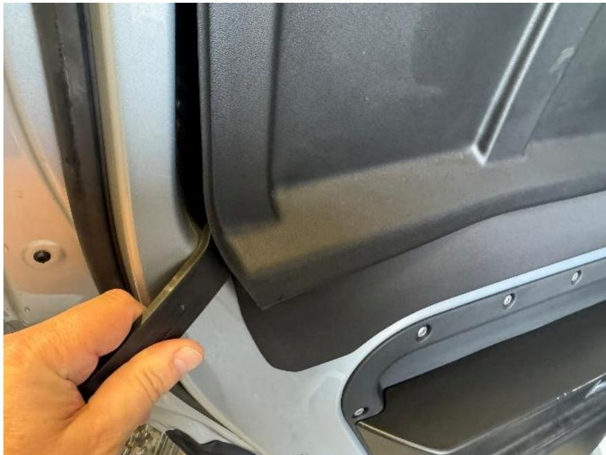
When you have revealed enough of the trim to be able to grab it with your hand, start to pull the trim away from the window frame. The Sikaflex adhesive is extremely strong so you may even tear the plastic window trim when removing it. Luckily Land Rover was less than exact when installing the trims so you'll probably find the adhesive barely touches some areas of the back of the plastic trim.
