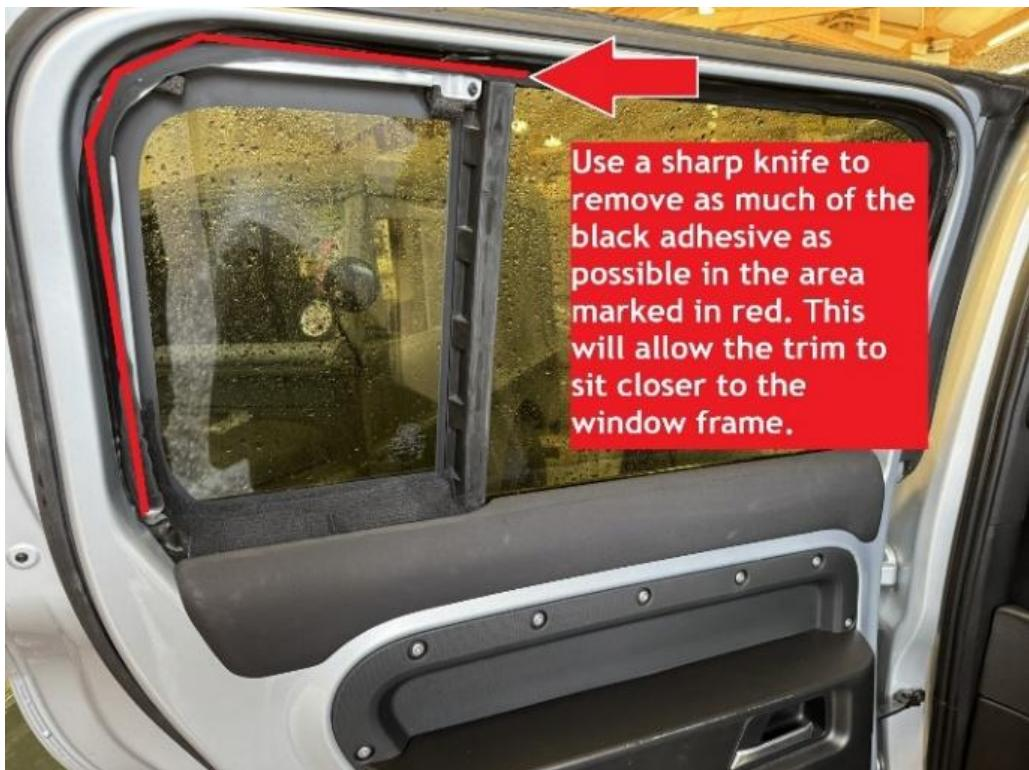
Ensure you reveal the fixing hole in the upper rear corner of the window frame where the single white fir-tree fastener on the new window trim surround will locate.
