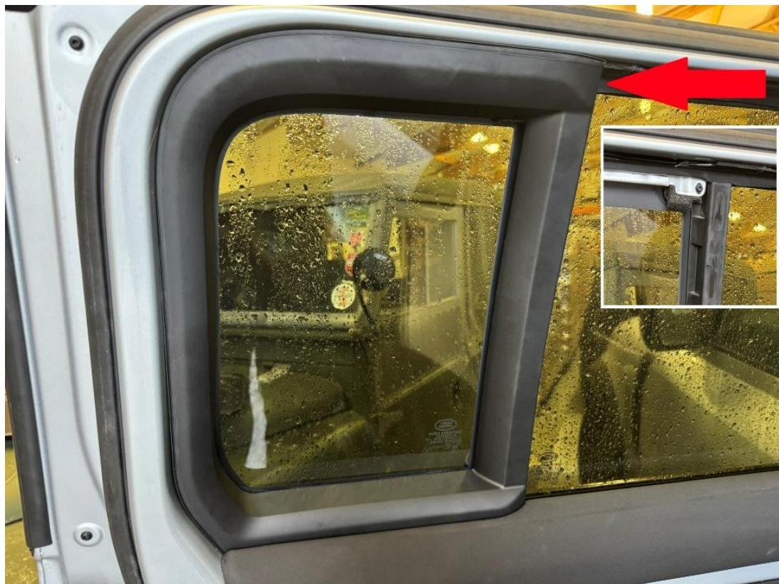
Fit the trim into the aperture. Be sure to locate the front vertical edge of the trim into the narrow window channel arrowed in yellow first. Now push the trim far enough back into the channel until you can locate the fir-tree into its fixing hole. Push on the corner of the trim panel until the fir-tree grabs the window frame.
