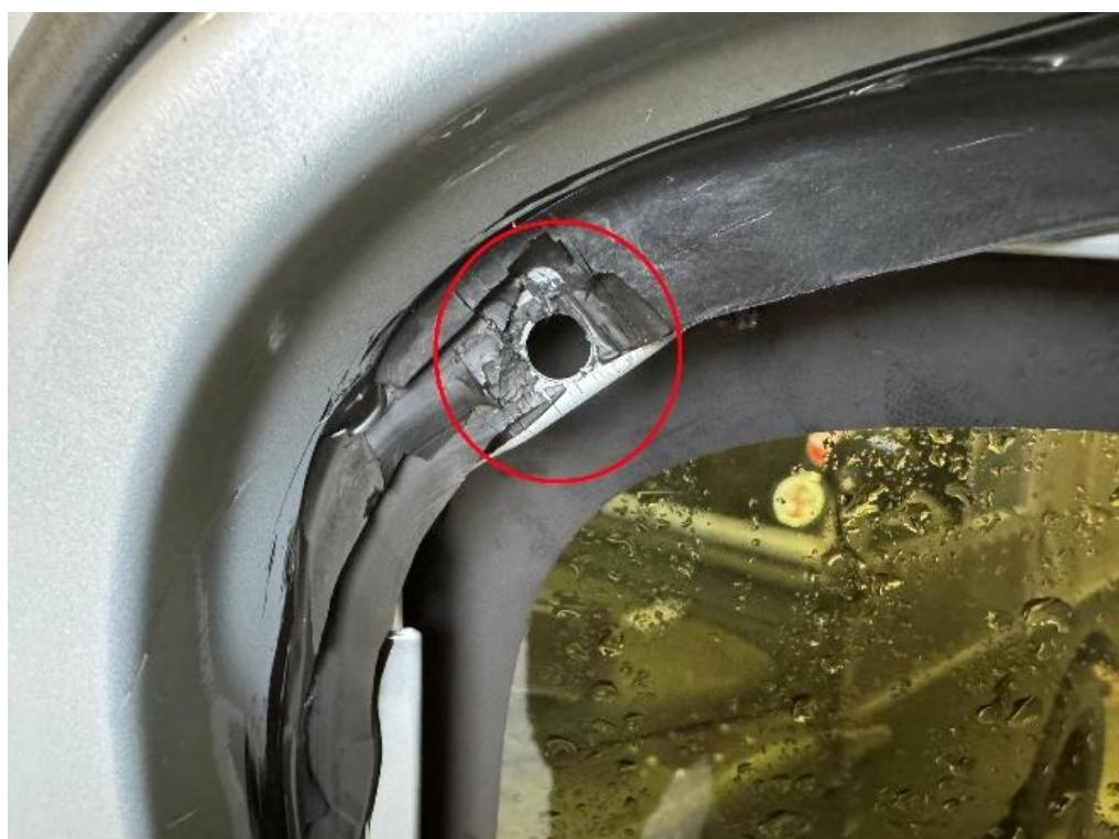
Make an incision in the centre of the fabric tape along the bottom of the window for the locating prong that you will find at the bottom edge of the new window trim.
