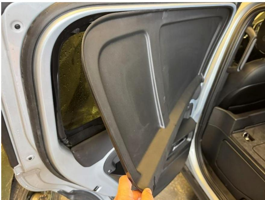
With the window infill panel removed, use a sharp blade to remove as much of the excess black Sikaflex adhesive as possible in the areas highlighted in red below. The more of the adhesive you remove the closer the trim will sit snug to the window frame. Take care with your knife to avoid scratching the paintwork.
