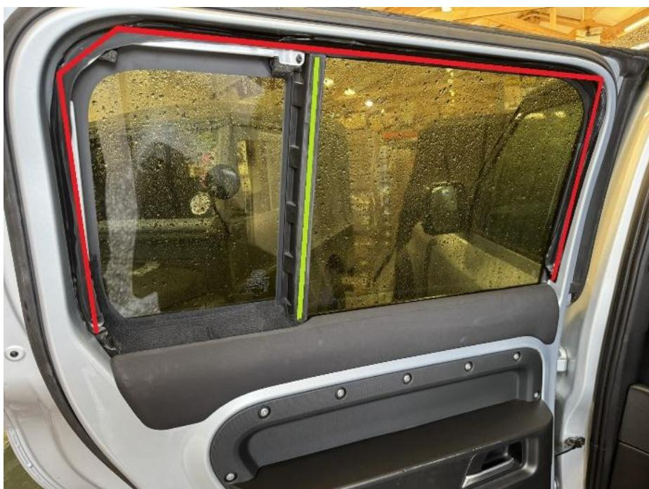
Use a trim tool to prise away one corner of the trim and start to peel it away from the window frame.
