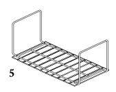
Turn around the table again, and screw the last two C screws to the backside of the two lamellas.
