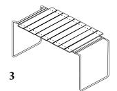
When the steel base and tabletop are put together, screw the last tw lamellas on with the B screws
