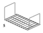
Turn around the table again, and screw the last two C screws to the backside of the two lamellas.
