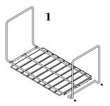
Place the table top downwards on a carpet or another surface that does not scratch the lamellas. Put the steel base and table top together with the A bolt, washer and nut.
