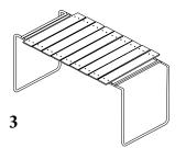
When the steel base and tabletop are put together, screw the last tw lamellas on with the B screws
