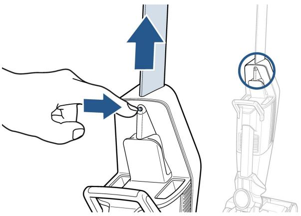
Pull up on handle while pushing blunt tip object into small opening to remove
