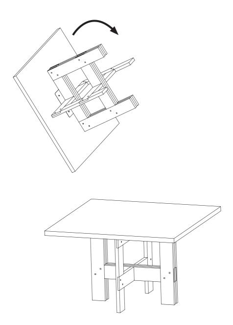
Start by placing the trestle section D perpendicularly to part C.
