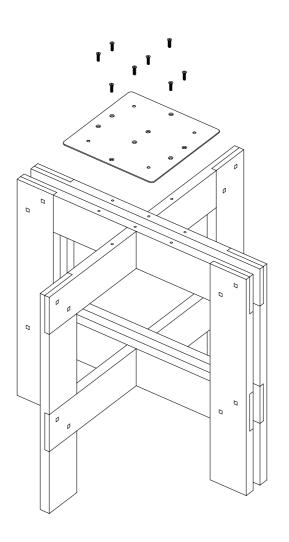
Mount the trestle upside down with attached metal plate B to the tabletop A. Fasten metal plate B to the tabletop with screws F using the allen key I.
