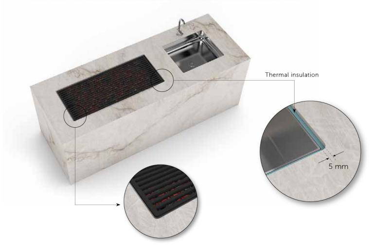
ELEVATED slabs withstand very wide temperature ranges and offer high heat resistance. Under the parameters of the ISO 10545-8 standard (determination of linear thermal expansion coefficient; see technical section of this catalogue), countertops created with Level slabs undergo controlled expansion with no impact on their mechanical strength, and they can therefore also incorporate grills and barbecues.
