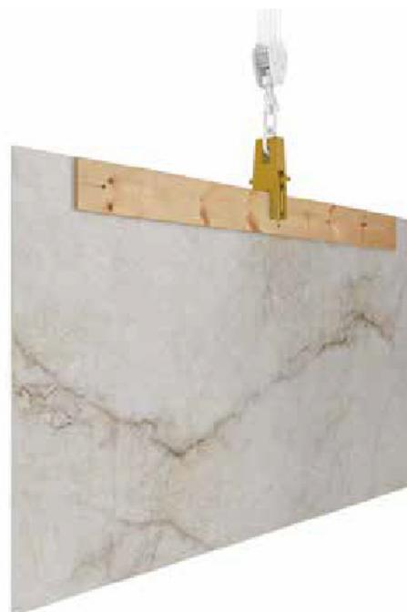
If a double **clamp** is not available, a **single** one can be used, enlarging its contact point by inserting a strip of wood of 300x20x2 cm. This is necessary to rotation or twisting of the slab, which could cause it to break.
