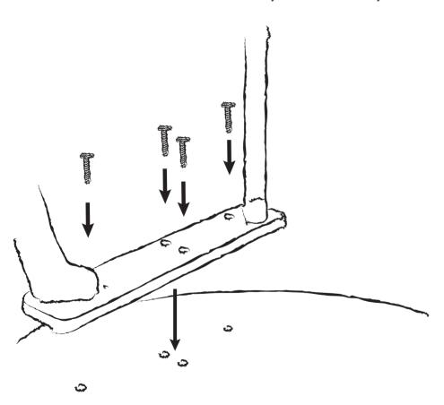
After this, the slats are placed between the leg ends and the end screws, which pass through both the leg end and the slat, are inserted without screwing them in.
