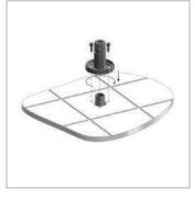
3. Position the spout outlet over the bath before tightening the grub screw.
