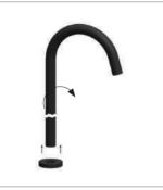
Slide the cover plate down over the base plate once the floor bolts have been tightened.
