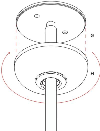
**Step 10:** Gently squeeze the protective paper and remove from canopy cover. Discard.
