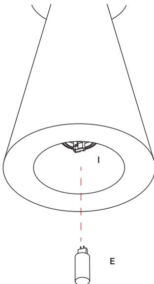
**Step 12:** Screw the diffuser (F) into the glass holder in the shade (I). Turn the power back on at the main fuse box or circuit panel you disabled before installation.
