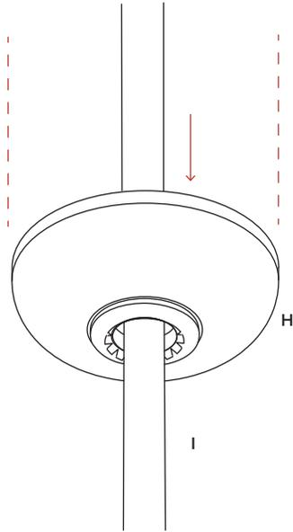
**Step 6:** Secure the brass stem to the canopy base (G). Rotate the stem clockwise to secure firmly in place.
