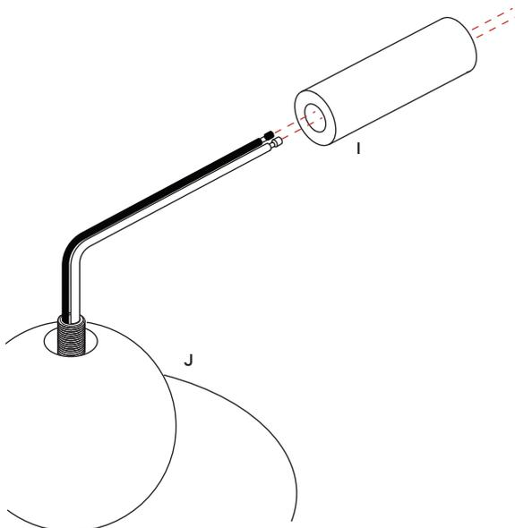
**Step 4:** Secure the stem (I) to the shade assembly (J). Rotate the stem clockwise to secure firmly in place..
